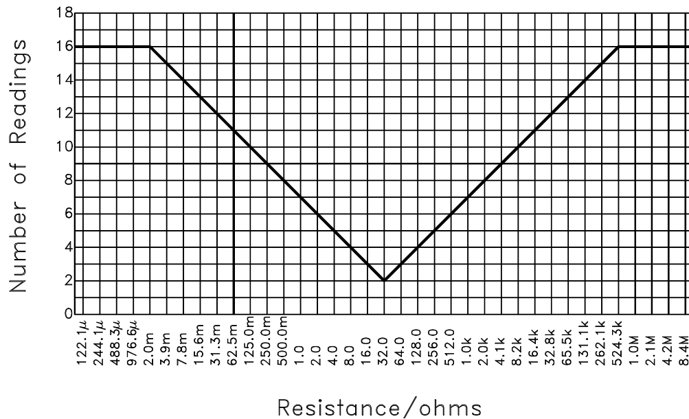
Figure 2-2. The number of measurements averaged in high-resolution mode varies from 2 to 16 and depends on how far from the base value of 32.767 Ω the resistance lies. Non-integers on the y-axis are rounded down in this graph.
